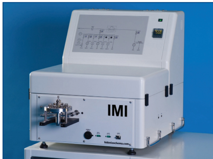
Figure 1: The IMI-HTP high pressure sorption analysis instrument.
